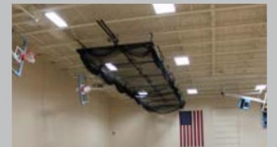
MODEL 4080BL BOTTOM LIFT MULTI SPORT CAGES are electrically operated sports cages that suspend from the ceiling • The bottom of the cage netting is automatically lifted to the top frame, eliminating the need to manually drape the net over the frame before lifting • Nylon straps hold the top frame at a preset height above the floor during use • Double cable spools uniformly pull up each side of the lower cage batten frame to within 1'- 9" of the structure.
